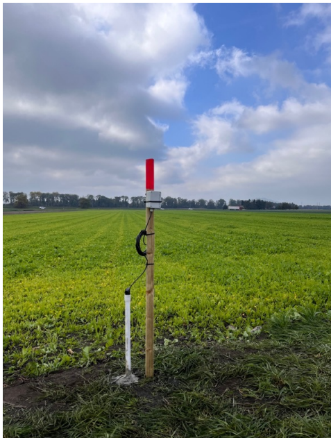
In situ soil moisture sensor measuring volumetric water content
